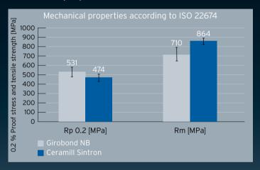
Ceramill Sintron greatly surpasses the strength requirements of ISO 22674 for Class 4 alloys (Rp 0.2: 360 MPa).
